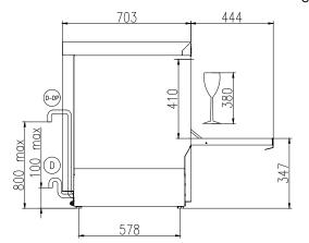
CWII = Cold Water inlet I (cleaning) D = Drain XD = Detergent connection
